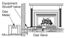
Figure 42 - Checking Gas Joints for Natural Gas Fireplace
